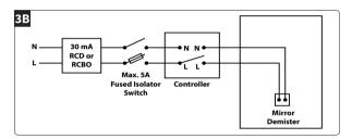
Alternatively they can be controlled by an independent controller that provides power on demand.
